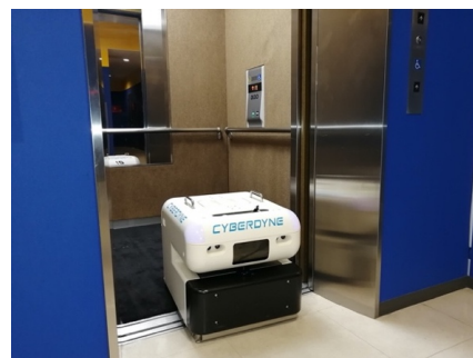
CL02 riding on elevators automatically
