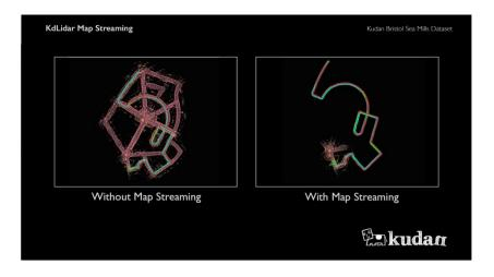
As you can see in the video, the system only loads the necessary part of the whole map depending on the vehicle's location. As the vehicle continues to move beyond the current map, the system predicts and fetches new sections of the map and unloads parts of the map that are no longer in scope to optimize memory usage.
