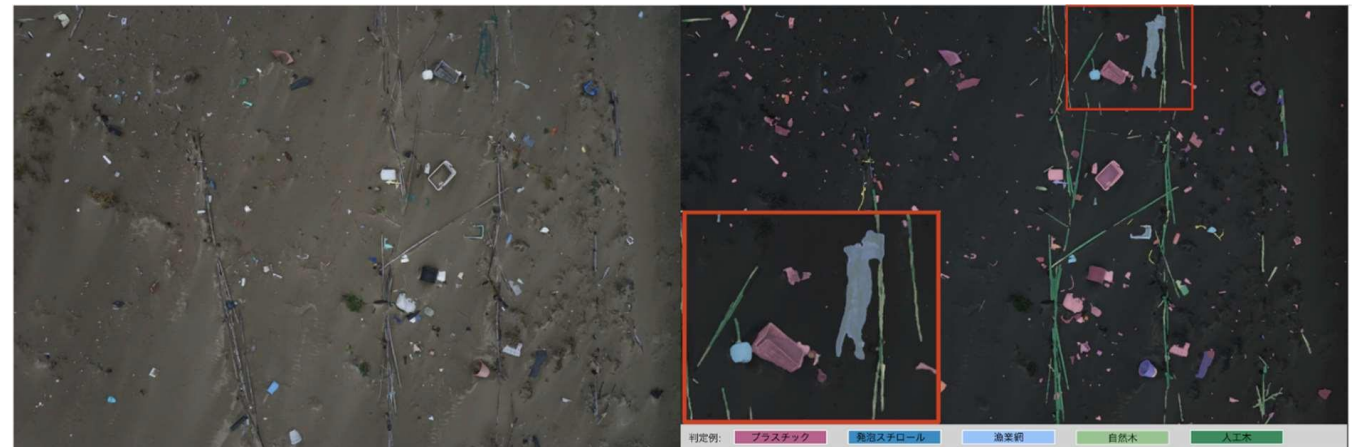
Using marine litter analysis AI to analyze the distribution and quantity of litter (Image taken (left), output of marine litter analysis AI (right))
