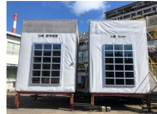
Test of transparent solar panels for use as windows
