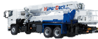
The AT-530CG boasts of the highest platform height and the largest working radius in Japan
