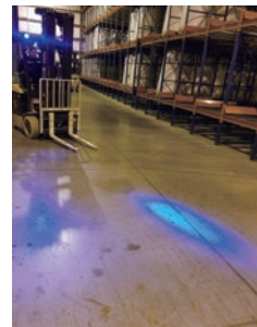
Forklift fitted with blue light to give advanced notice when a forklift is approaching
