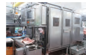
WANDAS Mini Mark II automated pork shoulder deboning machine
