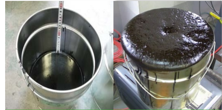
Mible-eco (generic term: foamed asphalt mixture)
