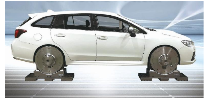
Actual vehicle tests with In-Tyre-House dynamo
