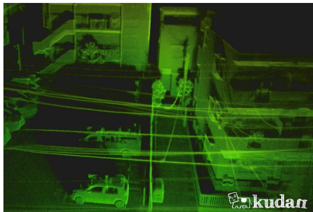
Kudan Lidar SLAM enables the accurate construction of 3D information that is the basis for the metaverse, the digital twin of space
