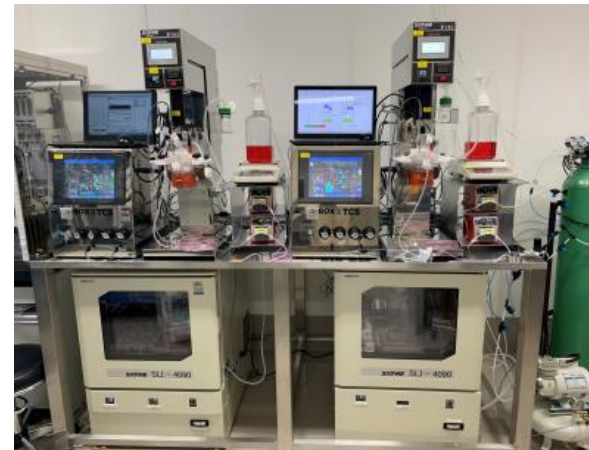
Proprietary, automated 3D perfusion bioreactor system for eNK production
