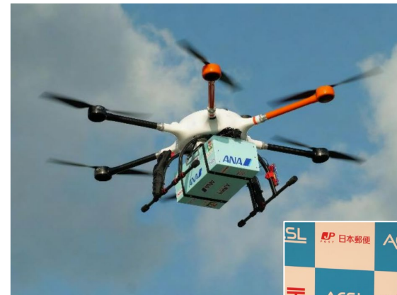
Actual cargo being transported in a medium-sized delivery drone demonstration with a 5 kg payload
