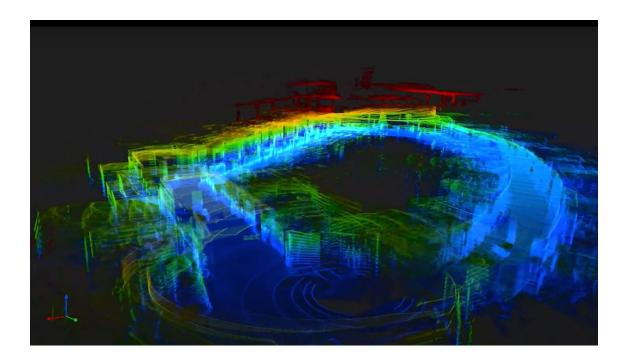
As you can see, when the robot completes the first loop (at ~0'17), it triggers a loop closure, and the map was adjusted and optimized to enhance its accuracy. The result is a sharp, crisp, and connected point cloud.
