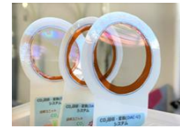
CO2 separation membrane as thin as 1/300 of human hair
