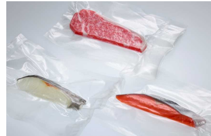
Food packaging film, an example of a nylon polymer application. Low oxygen permeability makes it suitable for food packaging.
