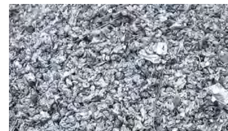
Iron recovered by magnetic separator
