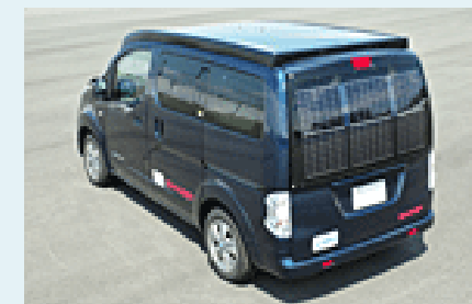
The e-NV200 electric vehicle with on-board solar panels
