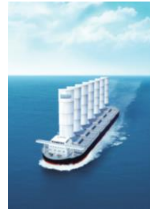
Image of a cargo ship with rigid sails
