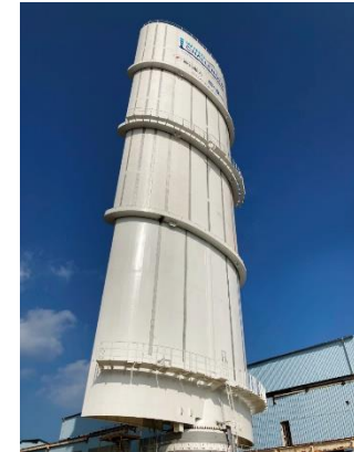
Rigid sail that can expand, shrink, and rotate automatically according to wind directions and speeds
