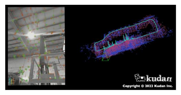
Our Visual SLAM enabled relocalization at random positions on the map and continued tracking. Also, our "Robust Against Change" mode together with the tilted camera mount allows robots to operate in environments where the scenery changes quite significantly over time. It can keep tracking on the map for a certain period of time even when 95% of the scenery is changed.
