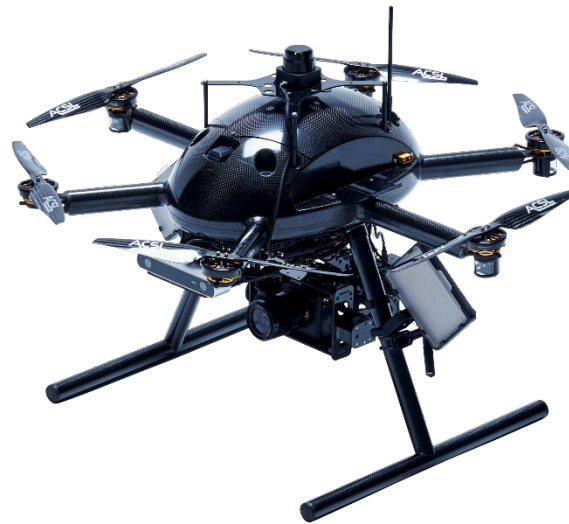
Chimney inspection drone
