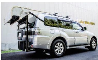
Vehicle fitted with road surface inspection system
