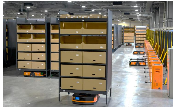
Automated guided vehicles (AGVs) operate in the goods-to-people (GTP) area
