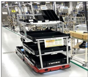
Automated transport AGV
