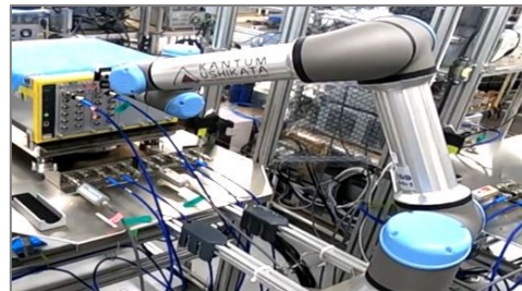
Inspection robot for T&M products
