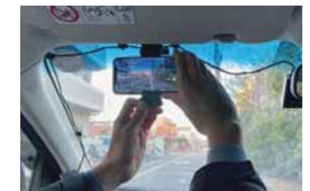
GLOCAL-EYEZ (smartphone-based road inspection system)
