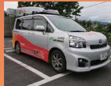
DX compatible road surface condition measuring vehicle SMART ROMEN CATCHER LY Jr.
