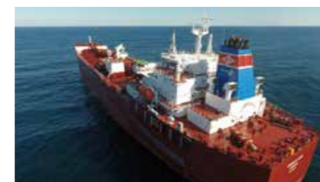
Chemical tanker with methanol dual-fuel main engine CREOLE SUN
