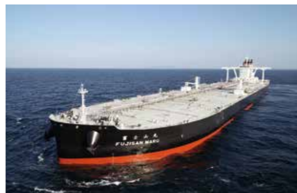
VLCC with SOx scrubber FUJISAN MARU (5th generation)
