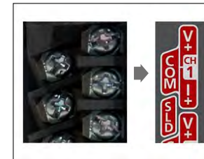
Print design illustrating the actual wiring
