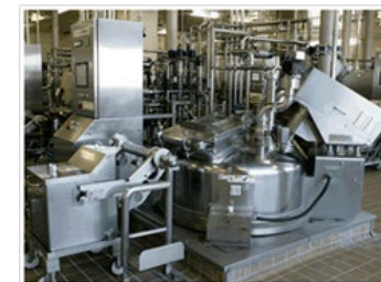
Byproducts used to power cooker (large steam oven) when making curry sauce
