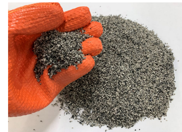
Waste carpet tile (crushed)
