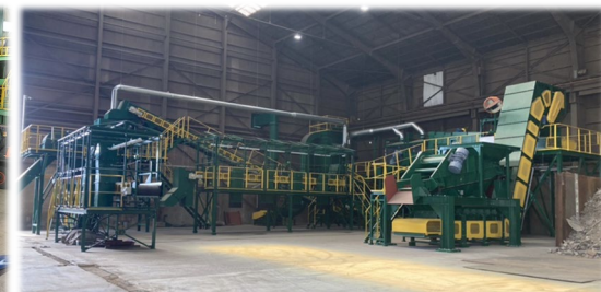
Sorting line for post-shear dust
