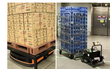
AGV for transporting pallets
