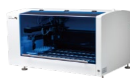
Histostainer-AT automated immunostaining device
