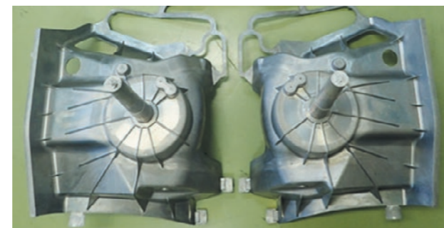
A vehicle body component (shock tower) produced by the HiGF method, Ahresty's unique technology 2 units/1 injection
