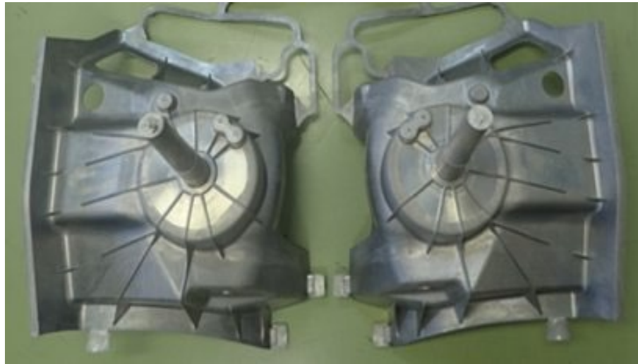
Shock tower adopting multiple cavities
