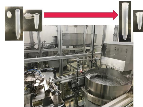
Automatic lid-closing robot This robot replaces employees’ routine and simple task of closing 2,000 lids per day.
