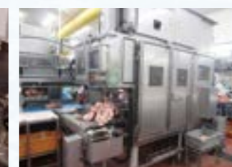
WANDAS Mini Mark II automated pork shoulder deboning machine
