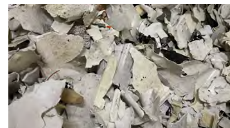
Mixed plastic separated from recovered urethane
