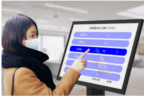
PCAP (projected capacitive) Hover Touch Display
