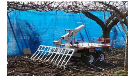
Branch collection with branch collection module
