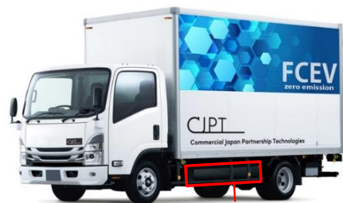
Large high pressure hydrogen tank
