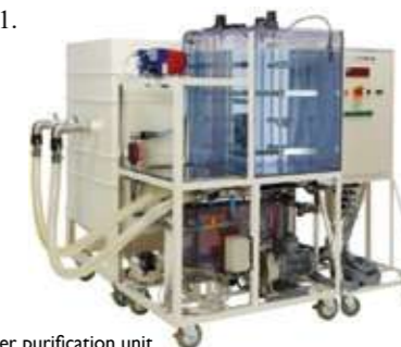
Flushing water purification unit
