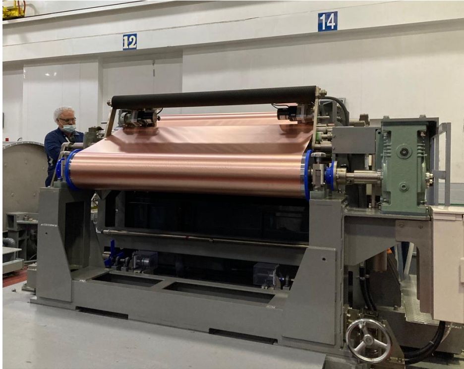
Photo: Production equipment of ED copper foil installed in Camden Plant, U.S.
