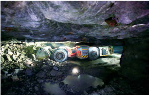
[GHH’s load haul dump suitable for narrow tunnels]
