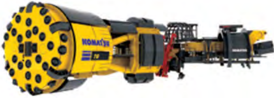
[Mining TBM for underground hard rock mine]
