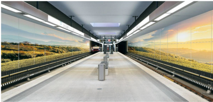
Image of subway platform walls finished with inkjet printing process
