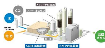
Conceptual image of a pilot plant in the SOEC methanation technology innovation business
