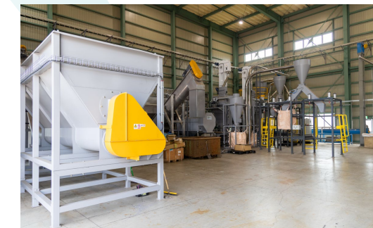
Using the resin sorting lines newly installed at REVER CORPORATION's Nasu Plant in FY2022
