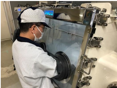
Glovebox for dismantling cells
