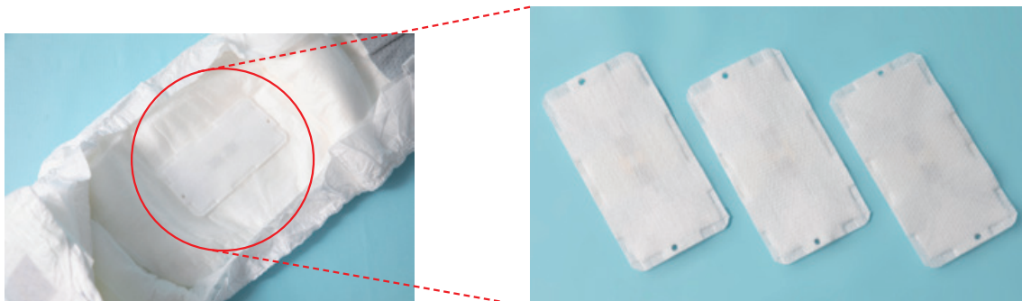
C-Letter, a Urination Detection Sensor
