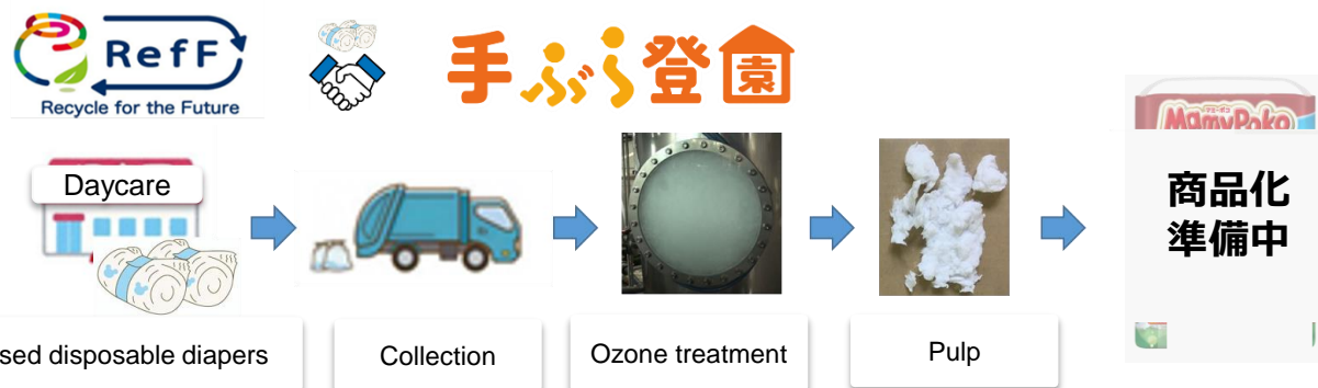
Process flow recycling from collecting used diapers from daycare facilities to creating new product
