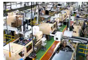
Resin part molding line
