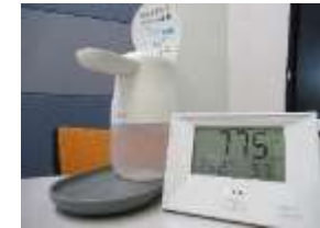
Installation of CO 2 concentration meter
