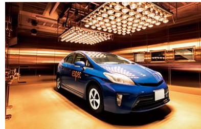
Drive-In Chamber for Vehicle Testing
