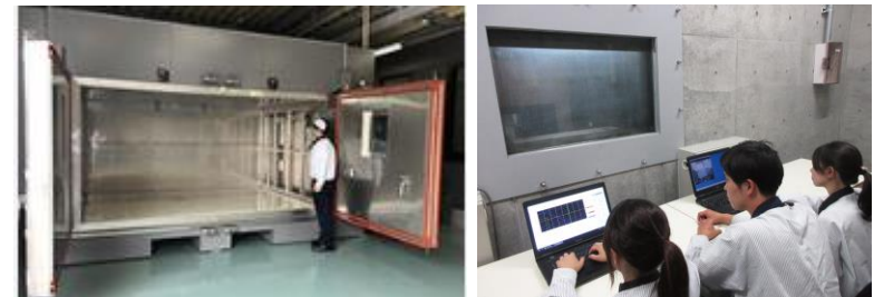
Capable of performing various safety tests for secondary batteries compliant with United Nations regulations and other standards Battery Safety Testing Center
