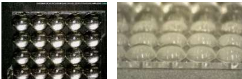
Thickness 0.5mm, \Phi 1mm 'shave a cell fly eye lens
