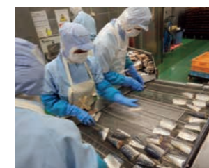
Work experience intern arranging fish fillets on a perforated tray on the grilled fish production line
