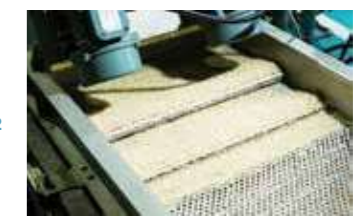
Pellets (material) recycled from used white trays
